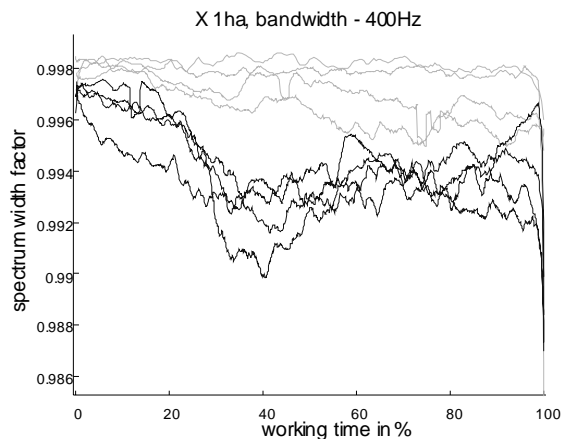
Fig. 8. Spectrum width factor of signal vibration acceleration in direction X in the bandwidth surrounding the first harmonic frequency with width of 400Hz.
